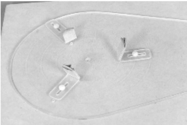
In some instances, it was found that the stops gave sufficient stability to the pot that there was no need to use the upper support, thus allowing for photographs with no visual intrusion into the pot mount.
