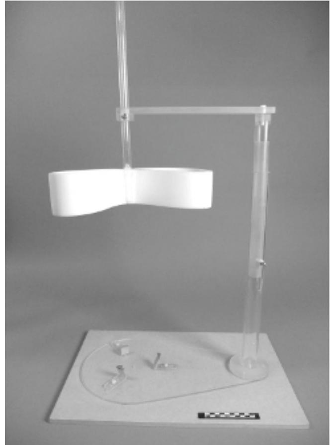
A horizontal arm of flat acrylic was bolted to the top of the column and extended over the position where the pot would be held. A ½" (12mm) acrylic rod was led vertically through a hole milled into the arm and a reinforcing block. An adjusting bolt in the reinforcing block allowed the rod assembly to be easily raised and lowered into the body of the pot.
