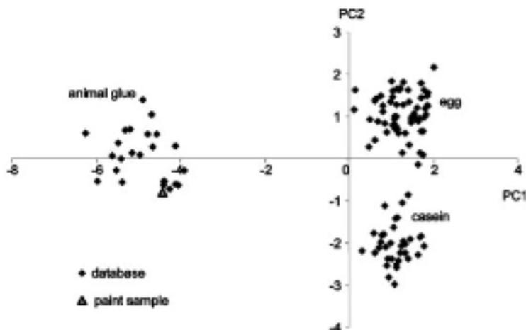
**Figure 4.** Pictured at left is an example of a plot generated using Principal Component Analysis (PCA). The plot depicts the relative amino acid percentages of glue, egg, and casein containing paint samples (non-aged and UV aged). Samples of unknown composition can now be compared to the cluster groups obtained using the PCA plot, assisting with the identification of proteinaceous materials in painted works of art.
