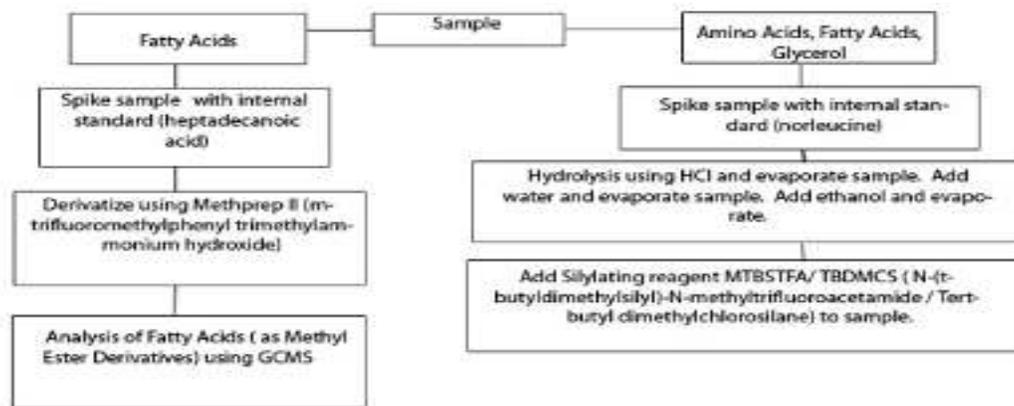
**Figure 2.** The flow chart below illustrates a protocol developed by scientist Dr. Maria Perla Colombini at the University of Pisa. This complicated protocol is designed to extract fatty acids, resins, waxes, amino acids, and polysaccharides from a single sample. One drawback to using more elaborate extraction methods is the size of the sample. Larger samples are often required for extensive protocols when preparing for analysis using GC-MS.
