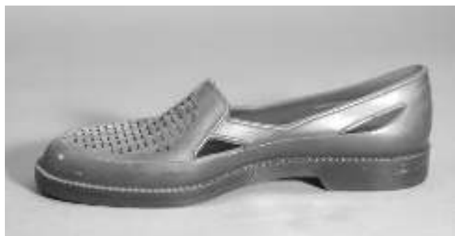
Fig. 2 Vinyl shoe from the Medicine and Science Division, NMAH. Migrated plasticizers form a sticky deposit on poorly ventilated areas of the shoe, such as the sole.
