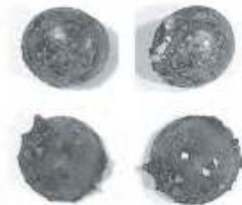
All of the studs developed bronze disease by the end of testing, which was confirmed by the presence of atacamite
