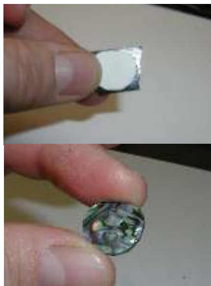
Shaped backing with oversized piece of veneer and final product
