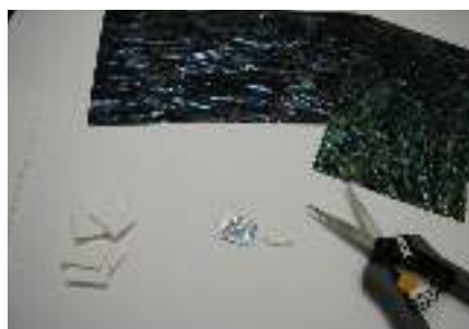
Shaped backing with oversized piece of veneer and final product
