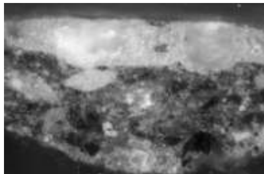
Figure 2a and b Moretto da Brescia, The Madonna and Child with Saints Hippolytus and Catherine of Alexandria . Paint cross-section from the red hose of Saint Hippolytus. Two large white inclusions can be seen in the uppermost red layer, which contains red lead and vermilion. 2a. Normal light, 2b. ultraviolet light.
