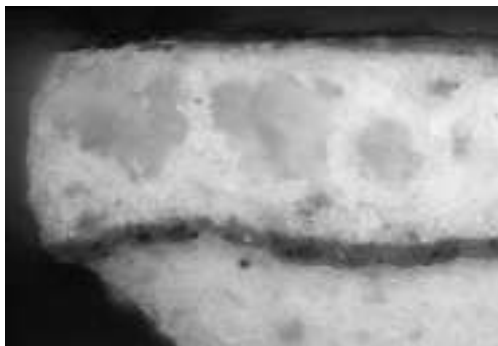
Figure 4 The Virgin and Child with Saint John, German School, 16th century, reverse of the Master of the Saint Bartholomew Altarpiece, Saints Peter and Dorothy (NG 707) . Cross-section from the highlight of the Virgin’s crown. Large translucent white inclusions are visible within the lead-tin yellow paint layer.
