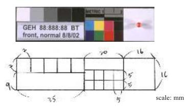
The gray scale and color scale (full-intensity only) patches are cut from a Kodak Q-13 Color Separation Guide and Gray Scale (small-20 cm), cat. #152 7654. (Note that as of January 2000, Kodak turned over manufacture and distribution of this item to the Tiffen Company, LLC.)
