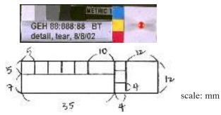
The gray scale contains the same 5 patches as the larger plate. Each patch is cut to measure 5 mm x 5 mm.
