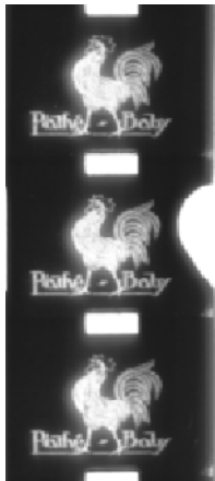
Figure 2: Pathé-Baby amateur film on acetate base with center sprocket holes.
