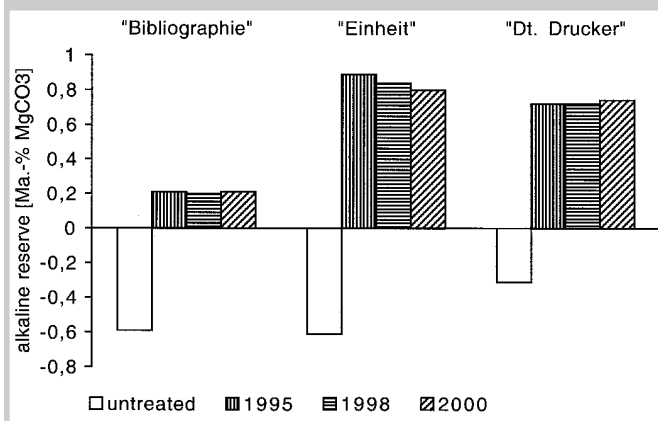
7 Alkaline reserve of the untreated samples, those deacidified in 1995 immediately after treatment and at sample-taking in 1998 and 2000.
