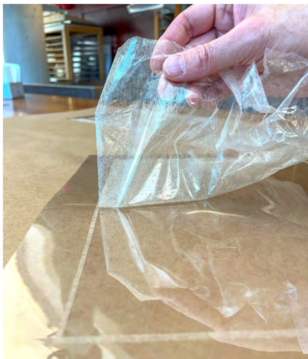
Fig. 3. The lining paper is a 2 gsm toned kozo tissue precoated with 5% Klucel G.
