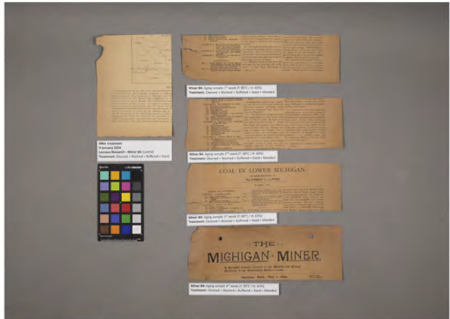
Miner B4 over four weeks of aging with Lascaux-WSP tissue, verso
