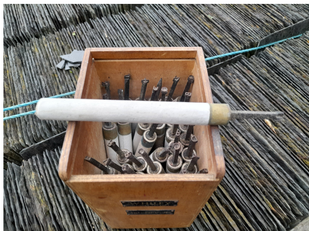
Fig. 7. Whiley handle letters with white-gray asbestos handles and brass ferrules. Courtesy of Paul Welters.
