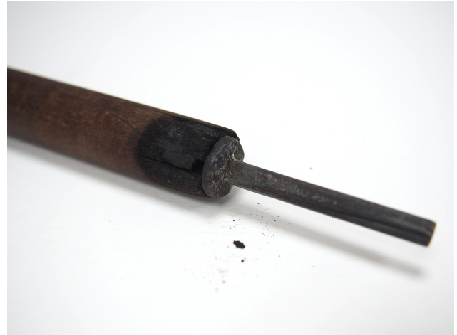
Fig. 2. A charred wooden handle that still holds onto the tool but drops unhelpful bits of charred wood onto the surface being worked.
