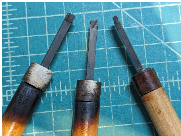
Fig. 9. Whiley Type B handles, of which the asbestos resin ferrules are damaged on the left and center tools.
