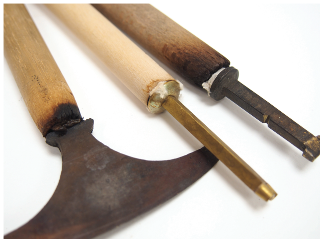
Fig. 3. Charred wooden handles repaired with glue (left), cotton wool (middle), and paper towel (right). The latter two wiggle gently, like loose teeth. The glued tool slides out of the handle gracefully as soon as it is heated on the stove. Parchment scraps are another classic hole-stuffing material. It is unlikely that asbestos would be used for this purpose: tool stuffing is usually a makeshift, in-the-moment solution, mid-tooling when the metal drops out but the job is not finished. Cotton wool is a common material to use for a wet pad to quench hot tools against and is therefore likely to be nearby. If in any doubt, identification should be made by someone with adequate training.
