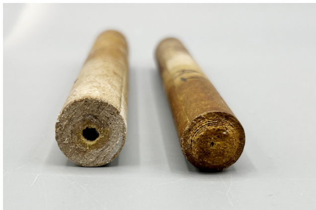
Fig. 12. Cockerell handles viewed from the end away from the tool: on the left, the asbestos handle appears sawn, and on the right, the uneven rolling is visible. Also note the large hole in the center on the left. Courtesy of Todd Pattison.
