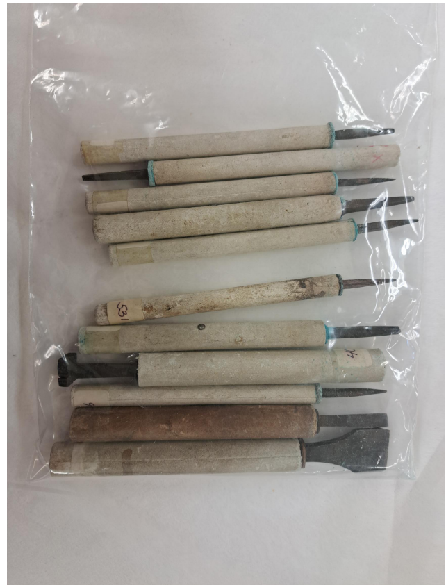
Fig. 11. A collection of asbestos-handled tools, many with corrosion on the cushions. They are all the white-gray type handles, except for the brown one second from right. Courtesy of Bronwen Glover.
