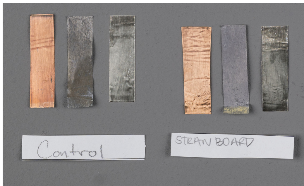
Fig. 8. Control coupon (left) and Board A strawboard coupons (right) after 29 days. Copper (left), lead (center), and silver (right).
