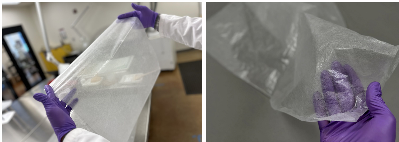
Fig. 3. “T2,” the main formulation of one layer of 3% Lascaux Acrykleber 303 HV, followed by two layers of 2% cooked Zen Shofu WSP.
