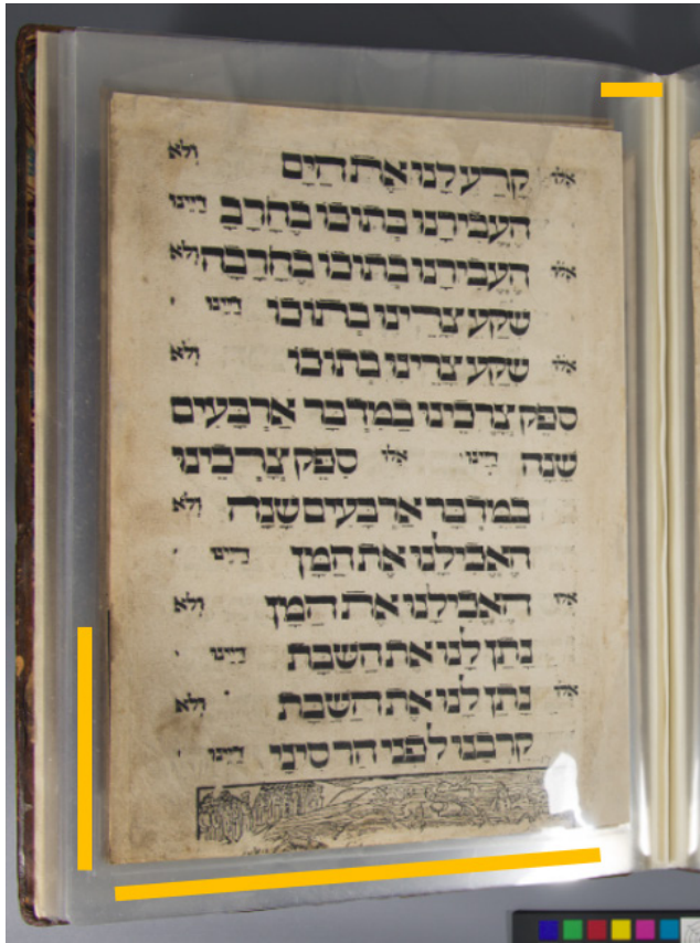
Fig. 13. Yellow lines represent outer ultrasonic weld lines.
