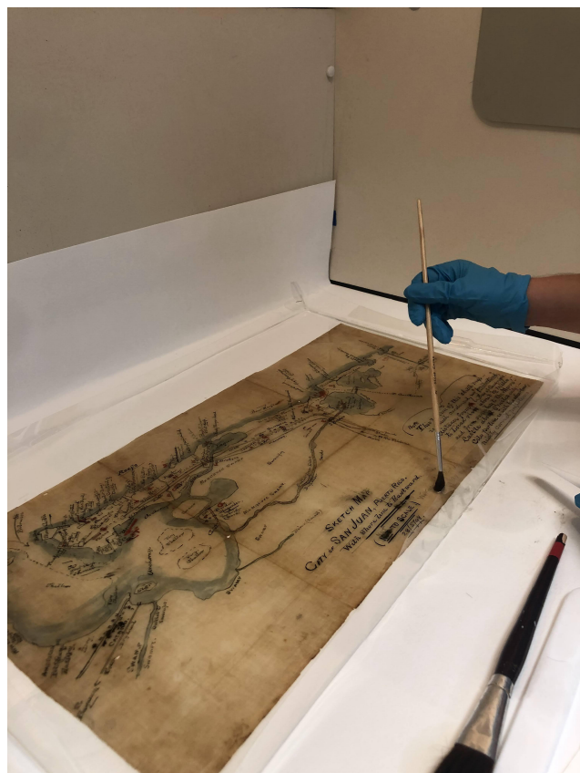
Fig. 7. The smallest map undergoing delamination in a disposable Mylar tray inside a fume hood.
