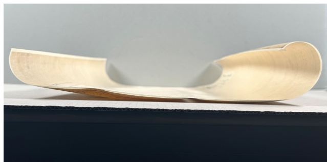
Fig. 4. Laminated and severely warped NARA record.
