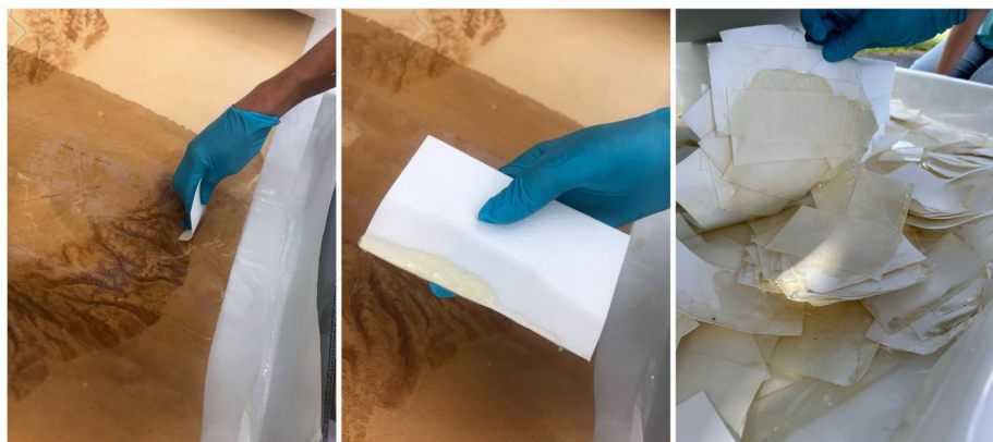
Fig. 13. Scraps of blotter used to manually remove softened laminate from the submerged object.
