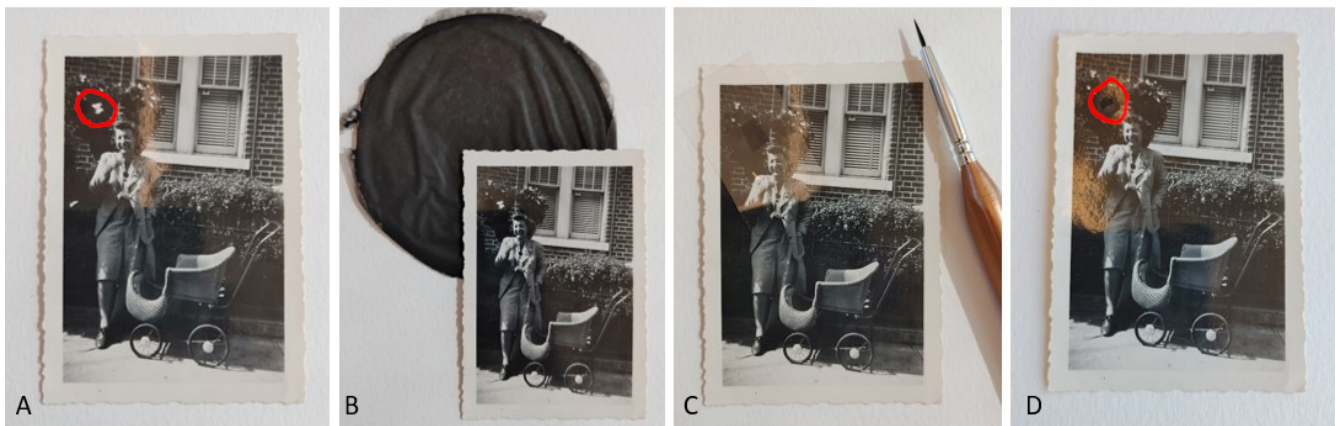
Fig. 15. First fill application trial on silver gelatin photograph. (a) Missing emulsion on silver gelatin photograph. (b) Matching a prepared nanocellulose film with the photograph. (c) 2.5% methyl cellulose placed on bare spot and nanocellulose overtop with Mylar. (d) Nanocellulose fill dried and excess removed.
