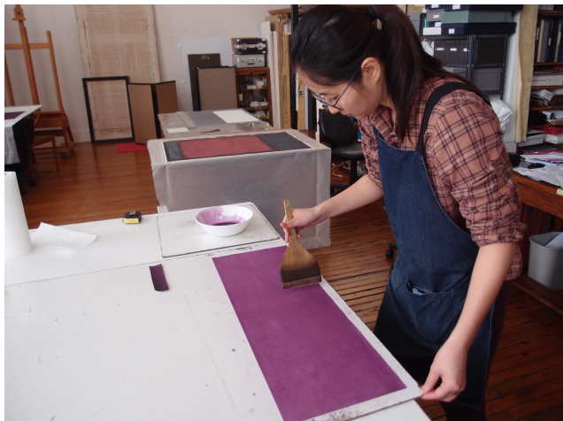
Fig. 6. Preparation of the new tacking edges. Coloring cold press Arches 90-lb. watercolor paper using acrylic paints.
