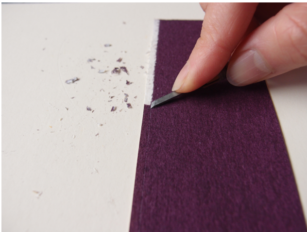
Fig. 7. Tacking edges were thinned in the pasting area to reduce thickness at the joints.
