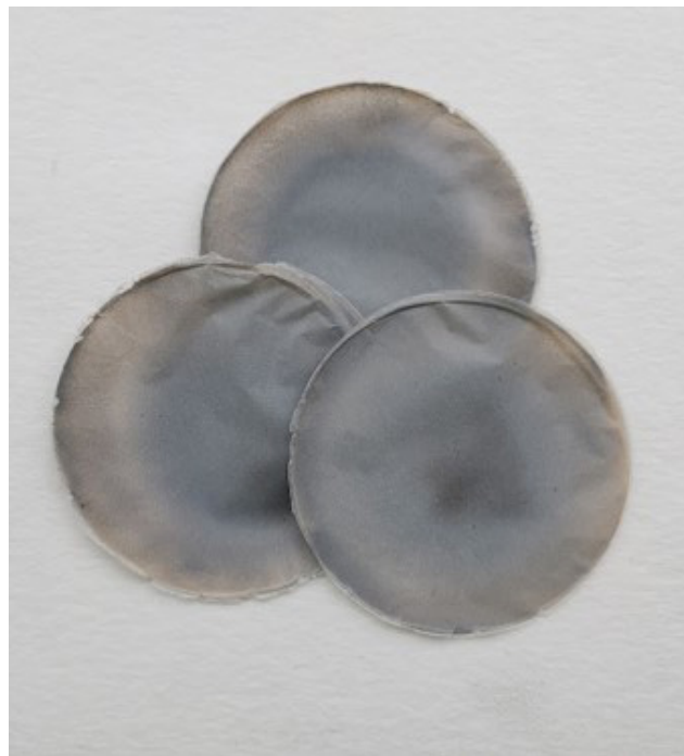
Fig. 7. Trial 5, air side, normal light. The less dense pigments rose to the top of the film. The final color appears more gray.
