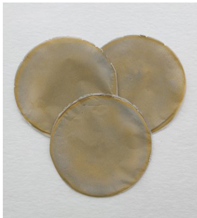
Fig. 8. Trial 5, mold side, normal light. The denser pigments sank to the bottom of the film. The final color appears more yellow.
