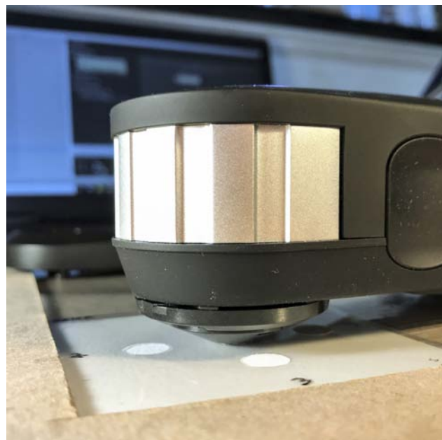
Fig. 3. Spectrophotometer and polyester overlay used to take color measurements of a paper sample.
