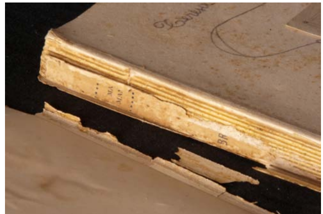
Fig. 8. Sewn, unsupported book bound in drawn-on covers from ETSEIB, UPC (Superior Technical Engineering School of Barcelona, Polytechnic University of Catalonia). Massive cracking along the spine material, board detachment, and friability of the unsupported sewing.
