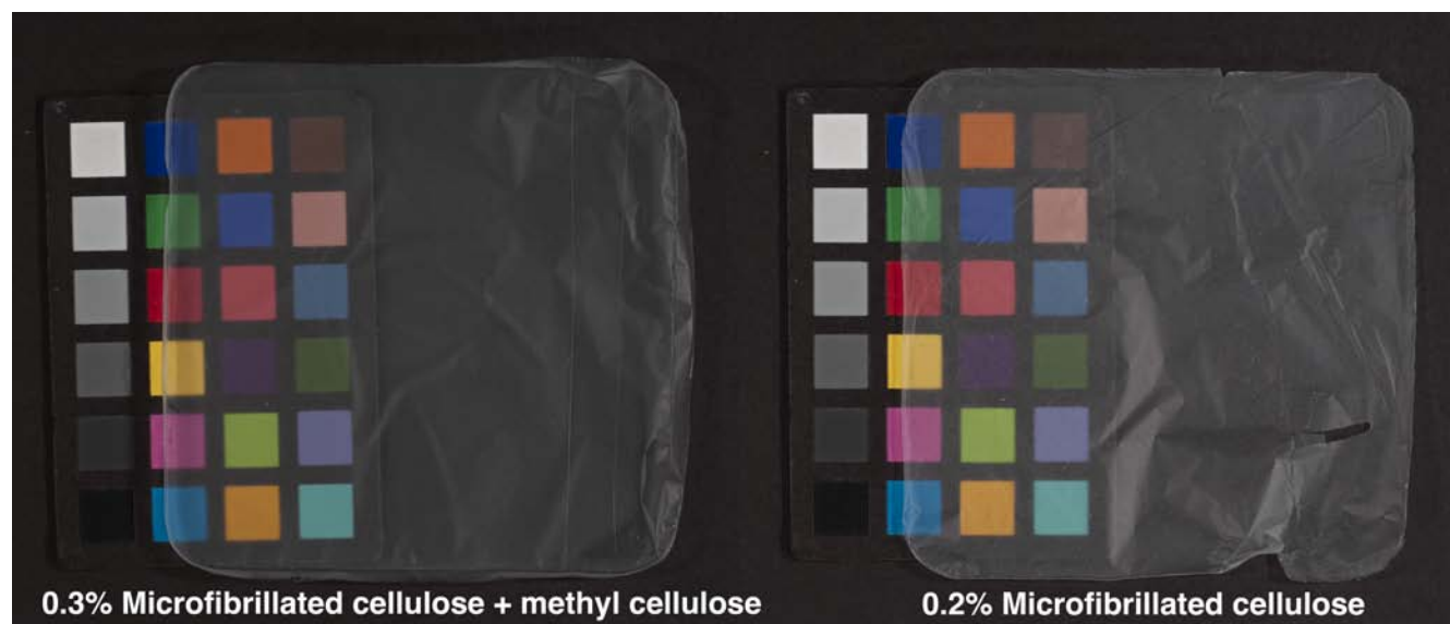
Fig. 3. A 0.3% MFC film prepared with methyl cellulose (left) exhibits slightly more transparency than a 0.2% MFC film (right).
