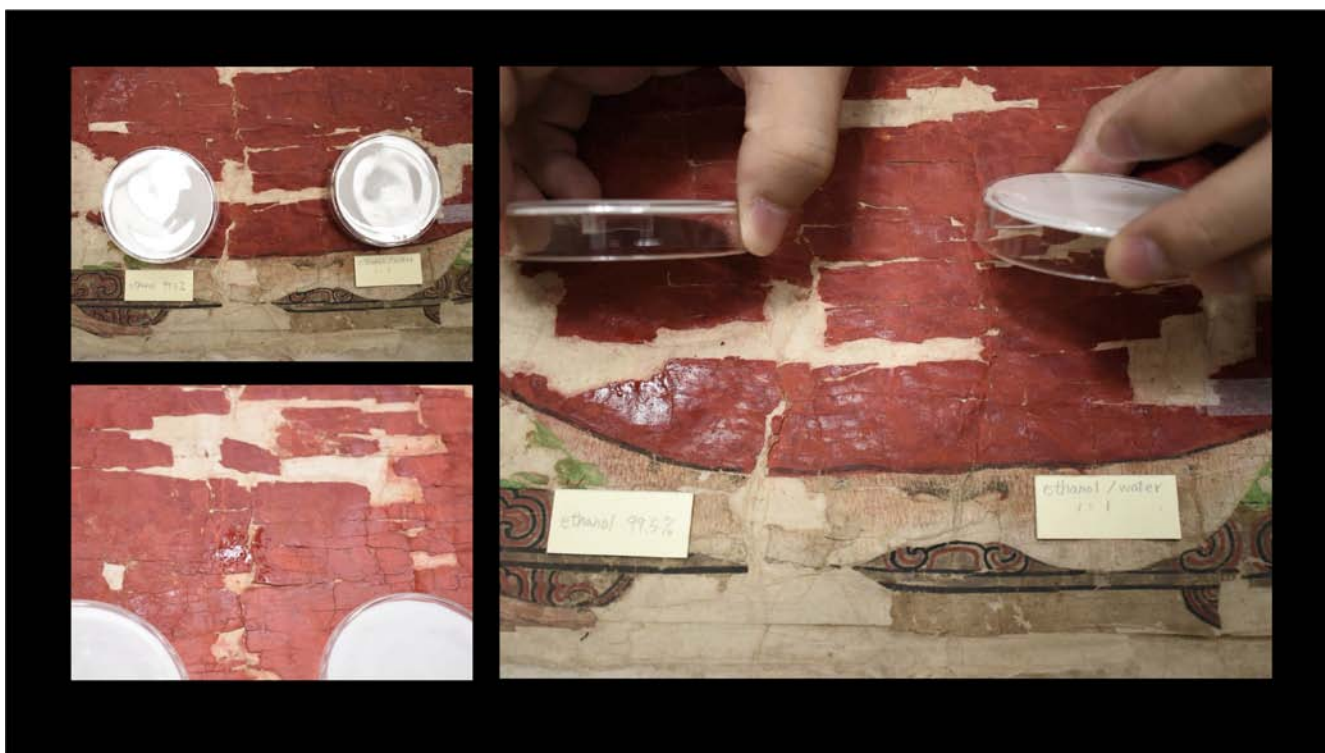
Fig. 6. Overpaint dissolving tests in different concentrations of ethanol. In the lower left and right, the paint is dissolved and glossy on the surface indicating the effect of ethanol.
