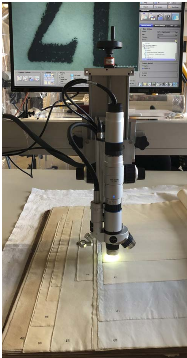
Fig. 3. A photograph detailing the setup of the HIROX digital microscope as handmade paper sample number 17 is examined.
