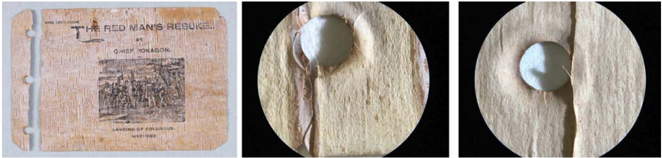
Fig. 8. The combination of vertical lenticels and the birch bark page flexing at the oversewing leads to splits in the page, as seen in the front cover of The Red Man's Rebuke (Special Collections Research Center, University of Michigan Library). Photomacrographs (15x magnification) show punched holes and a broken area within a lenticel of The Red Man's Greeting (AC85 P7565 893r, Houghton Library, Harvard University).
