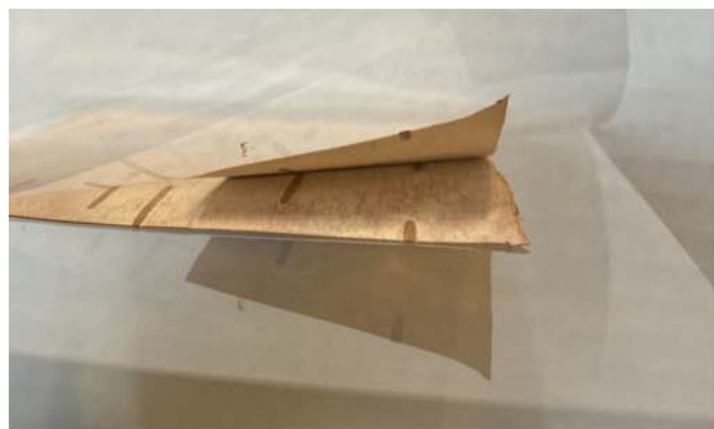
Fig. 15. The negative effects of using Mylar for storage with birch bark: delamination (left) and transfer of friable betulin layer (right).
