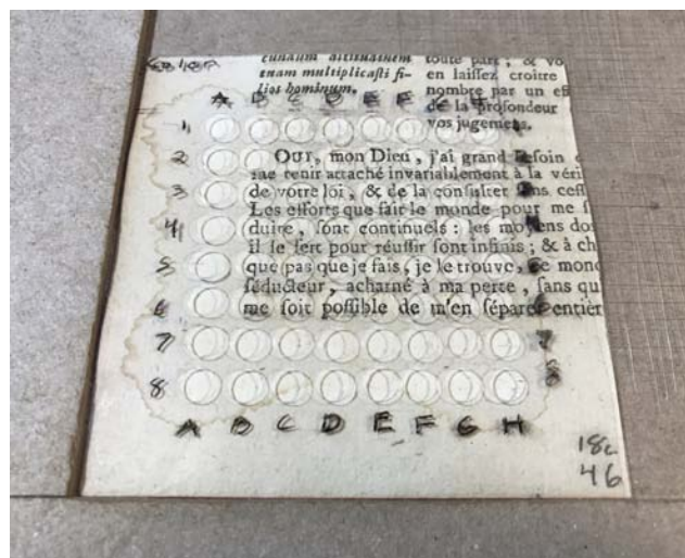
Fig. 4. Polyester film overlay with alphanumeric grid used to avoid the printer’s ink when taking color measurements of the antique gelatin paper samples.
