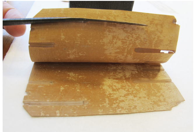
Fig. 12. Library label pasted to the last page of The Red Man's Greeting (AC85 P7565 893r, Houghton Library, Harvard University) causing the top layer of the bark to delaminate.
