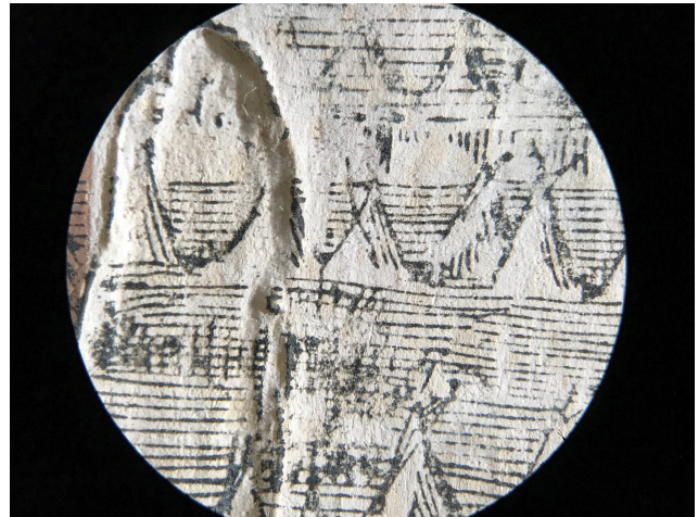
Fig. 2. Photomicrograph (15x magnification) of The Red Man's Greeting (AC85 P7565 893r, Houghton Library, Harvard University). An example of printing where the text sits only on the highest points due to the uneven surface.
