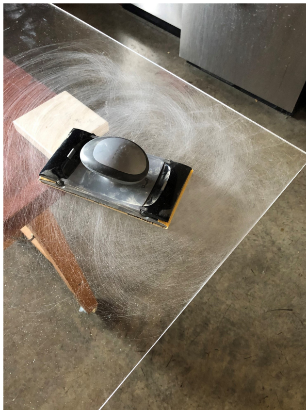
Fig. 8. Acrylic sheets getting sanded down with 60 grit sandpaper to prepare for lining.
