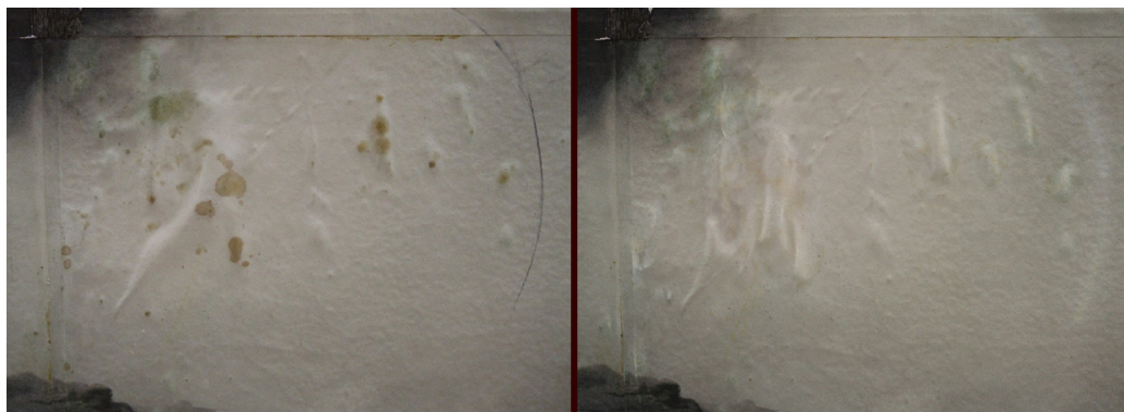
Fig. 8. Before and after stain removal with Laponite.
