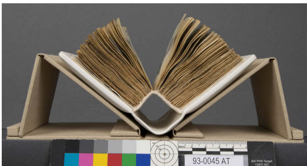
Fig. 16. Opening characteristics of HRC 10 after rebinding.
