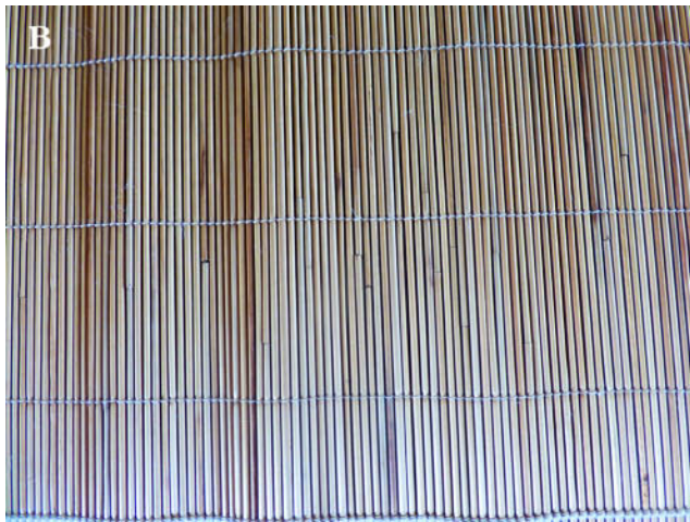
Fig. 23b. Detail of a kaya screen showing the random placement of laid support joins.
