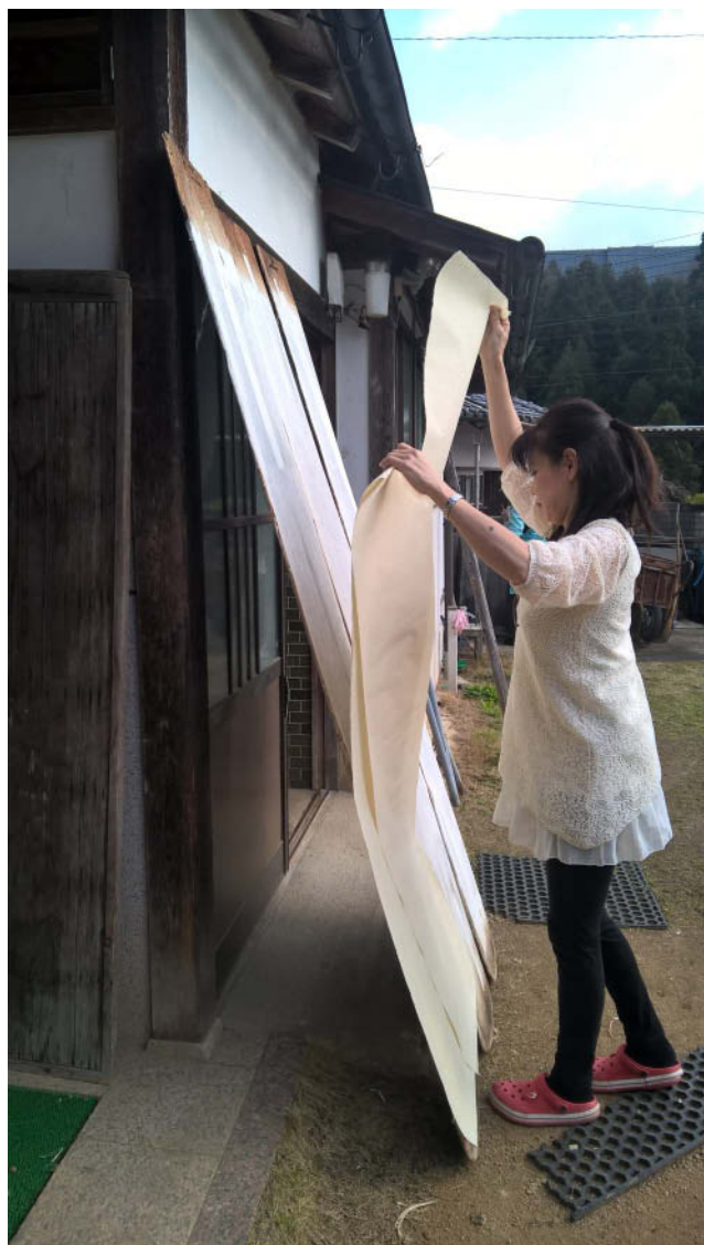
Fig. 16. Mrs. Fukunishi removing dried udagami sheets from wooden drying boards. Fukunishi Studio, Nara Prefecture.
