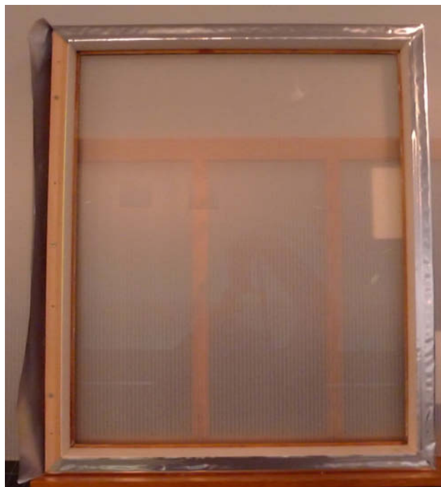
Fig. 15. Sealing strips wrapped around the sides of the basswood backing and attached to the back of the inner framed with 415 tape.
