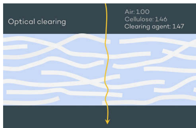
Fig. 4. A clearing agent provides a bridge of easier transition between the fibers of a disordered medium.
