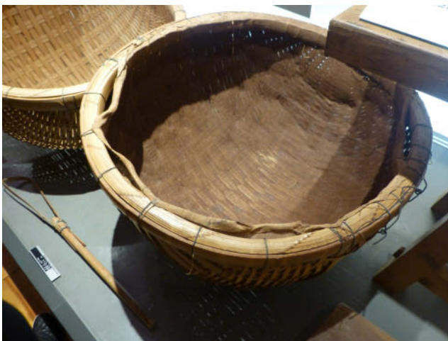
Fig. 19. A koburi basket on display at the Tōsa Wahi Musuem in Kochi Prefecture. The basket is used for the additional rinsing of fibers after they are beaten. This step is unique to papermaking in Kochi.
