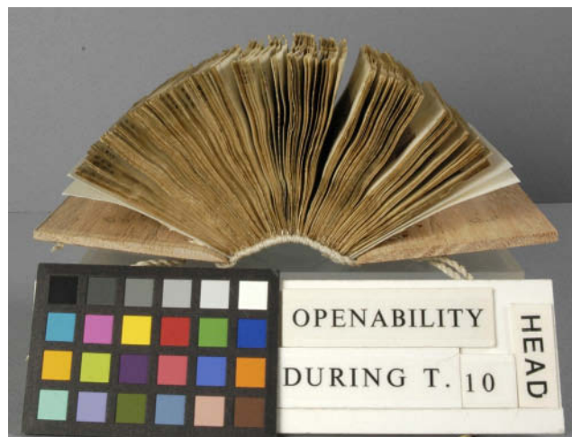
Fig. 5. Poor openability of HRC 10 after resewing on doubled raised cords.
