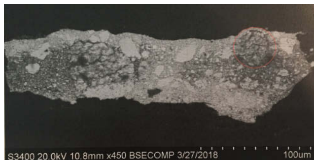
Fig. 9. Backscatter Electron photomicrograph of a sample of the ground from Portrait of Alphonse Maureau . The circled area is the location of possible lead salt formation.
