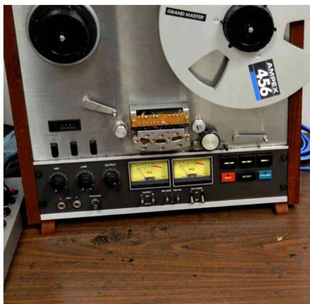
Fig. 4. 10-in. reel-to-reel player/recorder with head protectant shield removed for flaking magnetic layer to exit the machine. Note the flaked materials on the table. Credit: Roy Canizaro.
