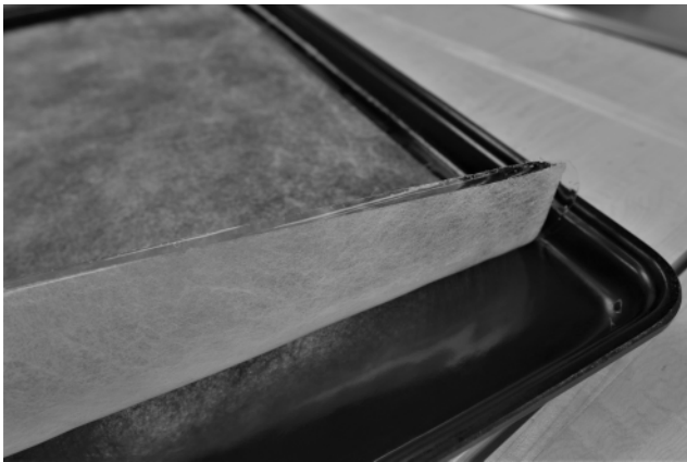
Fig. 6. The gellan gum is perfectly smooth on the tray side and large sheets are easily handled.
