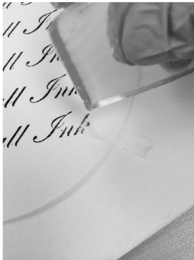
Fig. 3. Dry precoated tissue is laid in place and touched with gellan gum to reactivate the adhesive.
