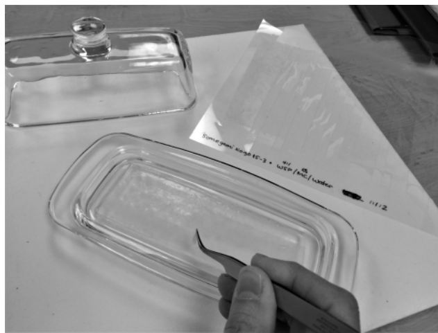
Fig. 1. A butter dish makes a convenient container for holding a sheet of gellan gum. Strips of water-sensitive adhesive pre-coated tissue lay on the gellan gum to reactivate the adhesive.
