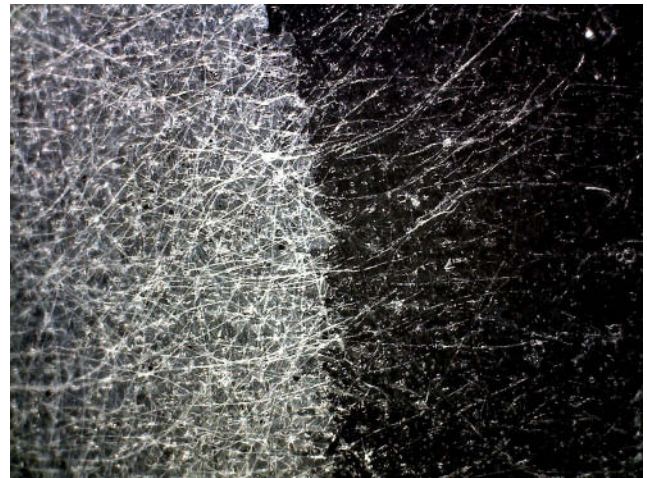
Fig. 9. A sample of BC Tissue over a black background (140× magnification). The left side is uncoated, and the right side has been optically cleared with Plextol B500.
