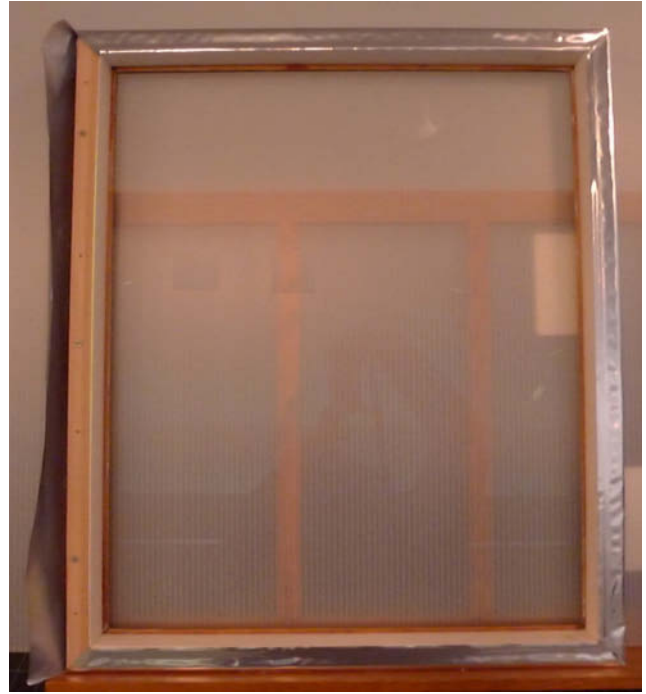
Fig. 15. Sealing strips wrapped around the sides of the basswood backing and attached to the back of the inner frame with 415 tape.
