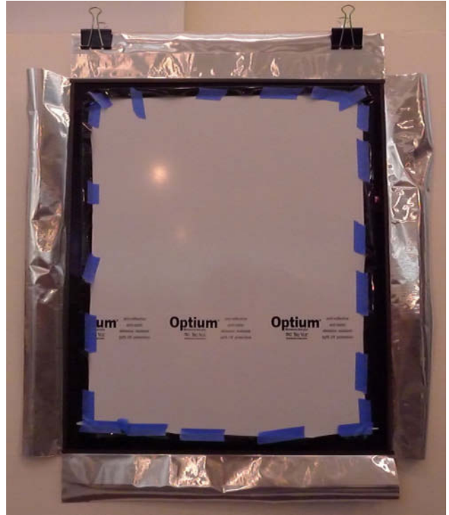
Fig. 12. All four sealing strips attached to the face of the Optium glazing.
