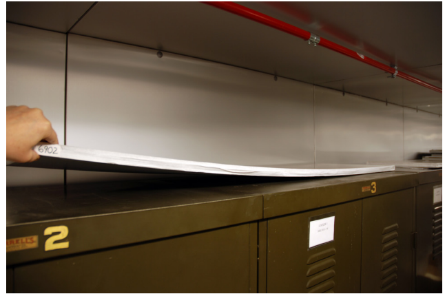
Fig. 10. Flexing of acrylic glazing.
