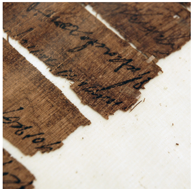
Fig. 11. Small fibers scattered due to static from acrylic glazing.
