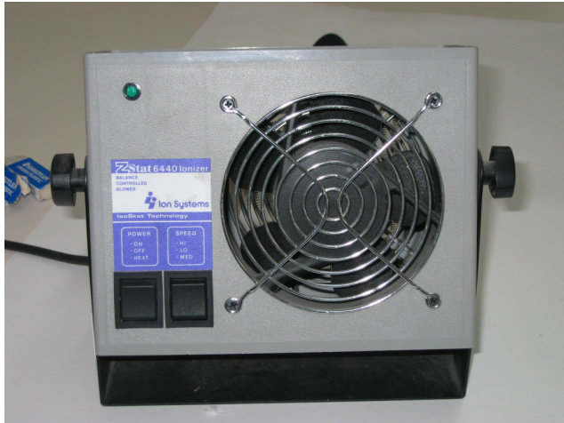
Fig. 9. Air ionizer used to reduce static when opening plastic housings.
