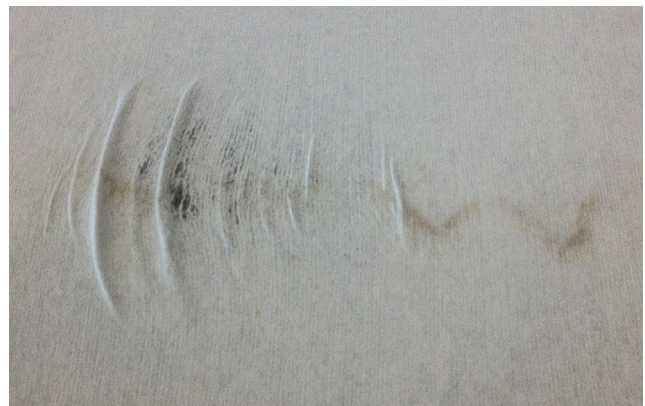
Fig. 3. Defibrillation occurring in TEK-Wipe from scrubbing.
