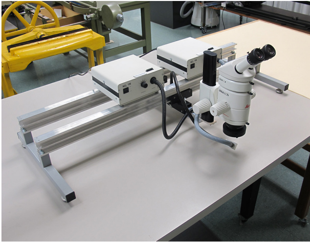
Fig. 1. Leica® Mz75 stereomicroscope in custom built bridge stand at the University of Hawaii Preservation Department Paper Lab.
