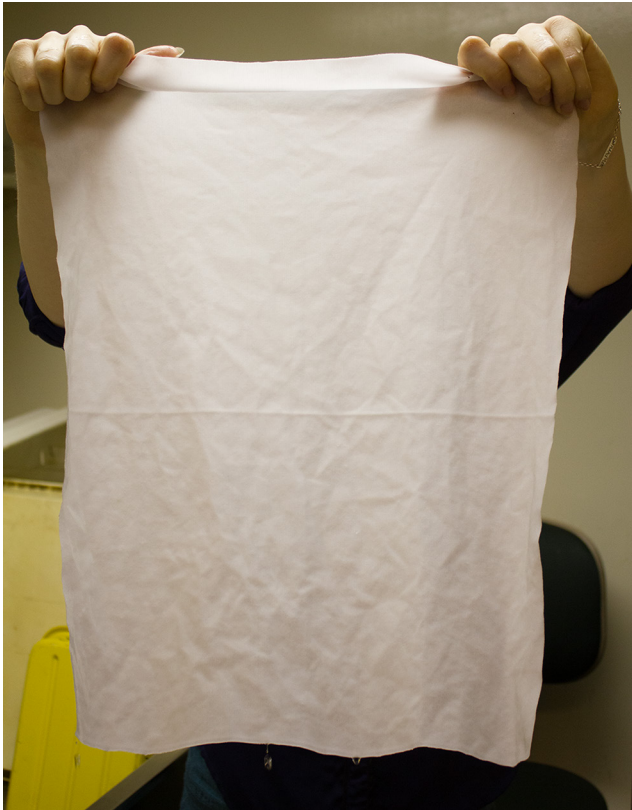
Fig. 6. TEK-Wipe can be lifted by one end when wet without falling apart; Courtesy of A. Kaspar 2016.
