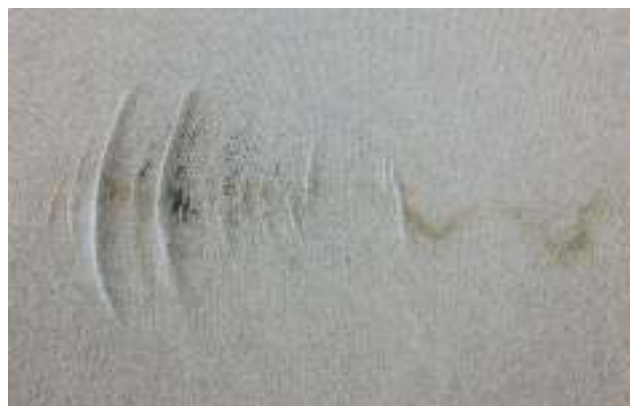
Fig. 3. Defibrillation occurring in TEK-Wipe from scrubbing.
