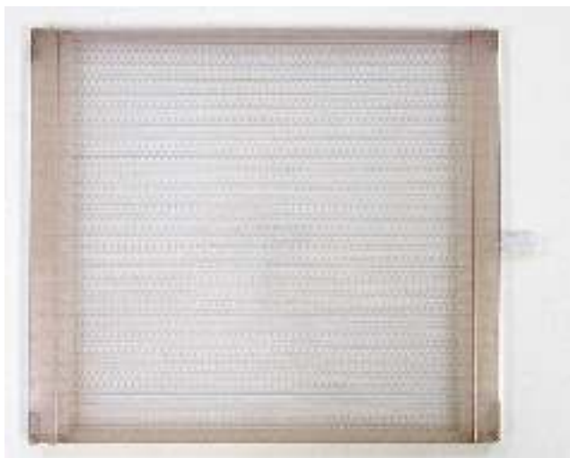
Fig. 26. Bottom of clear suction platen after completion.
