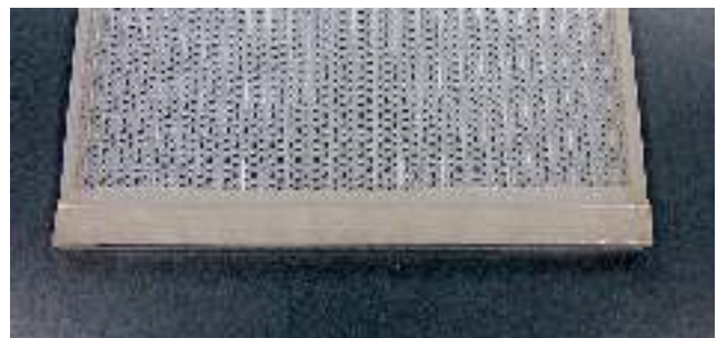
Fig. 24. A strip of Teflon tape is run across the two end caps on the bottom of the platen to create a seal.
