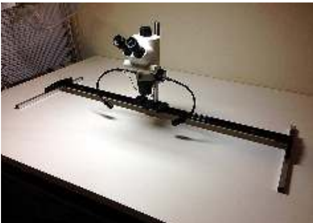
Fig. 9. Leica® S6D stereomicroscope mounted on adapted Glide Gear® Camera Slider with a used Nikon® focus mechanism.
