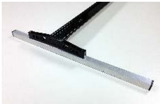
Fig. 22. Aluminum tubing mounted into the bottom of the detachable legs and installed back onto the track.
