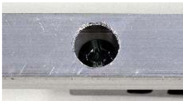
Fig. 21. Close up of the bottom of the aluminum tubing after mounting holes are drilled for screws.
