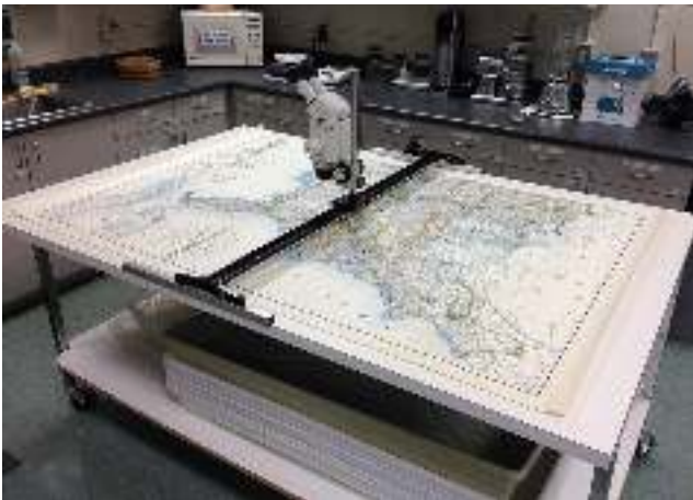
Fig. 8. Leica® Mz7s stereomicroscope mounted on adapted Glide Gear® Camera Slider with a used Nikon® focus mechanism.
