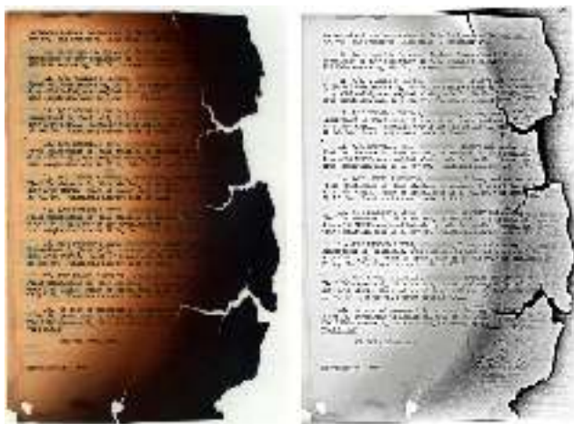
Fig. 1. Before and after image of digitized burned document using infrared photography and Photoshop enhancement. Photo courtesy of Lenin Hurtado, Reformatting Lab, Preservation Programs at St. Louis.
