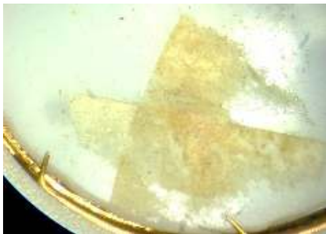
Fig. 7. Metal prongs on the verso of the bezel, holding the cover glass and portrait together.
