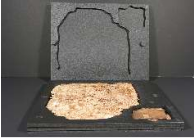
Fig. 9. Binding in its “sandwich” of archival foam board, outer layer of Volara, and inner layer of laser cut Volara; Courtesy of the authors.
