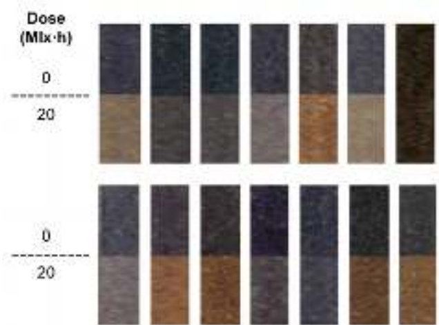
Fig. 3. Image of 14 dye-based fountain pen inks unexposed to light, and exposed to a dose of 20 Mlx·h. Sample ink strokes were prepared on buffered paper with a broad 3 mm wide fountain pen nib.
