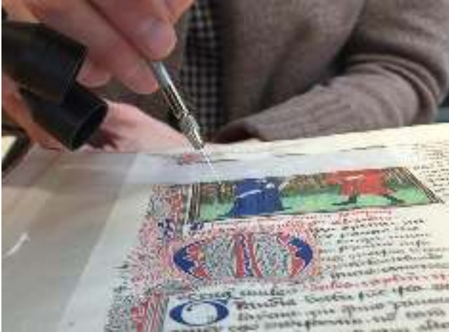
Fig. 11. Endontic absorbent paper points used for media testing. Conservator steadies hand with pinky finger on fiber optic light stem.
