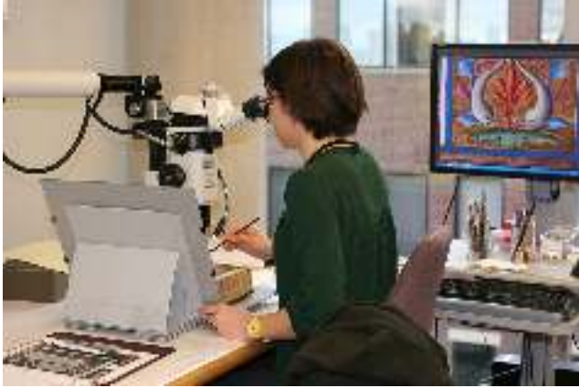
Fig. 1. One of two stereomicroscopy stations for consolidation. The floor stand makes this microscope ideal for large format materials.
