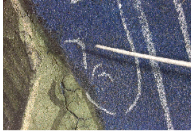
Fig. 12. Absorbent paper point in use at 15x, the magnification used for media testing. MS Typ Inc 2756. Missal. Houghton Library, Harvard University.
