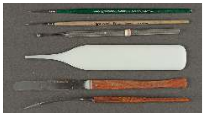
Fig. 17. Typical selection of hand tools in our consolidation process. Short handle brushes 4/0 to 5/0, round-ended dental tool, home-made shaped Delrin spatula, and spatula with extension of silicon-coated release Mylar.
