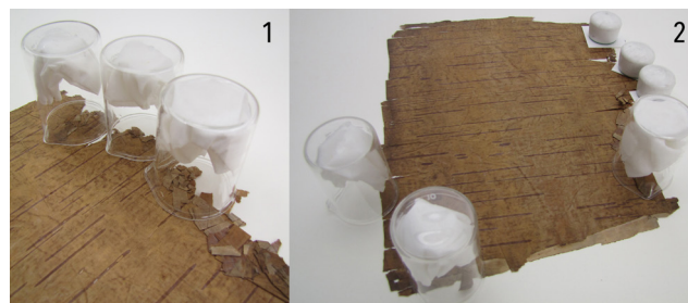
Fig. 10. (1) Solvent chambers made of inverted beakers with lightly methanol-dampened tek-wipe wadded inside and (2) the light weights and blotters used to plasticize and re-align bark layers while the solvent chambers worked elsewhere on the leaf. Full alignment often required multiple solvent vapor applications.
