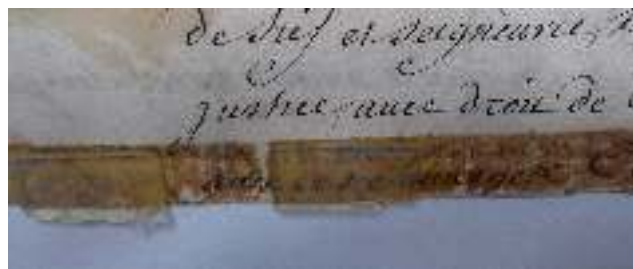
Fig. 1. Pressure sensitive adhesive stain before treatment.
