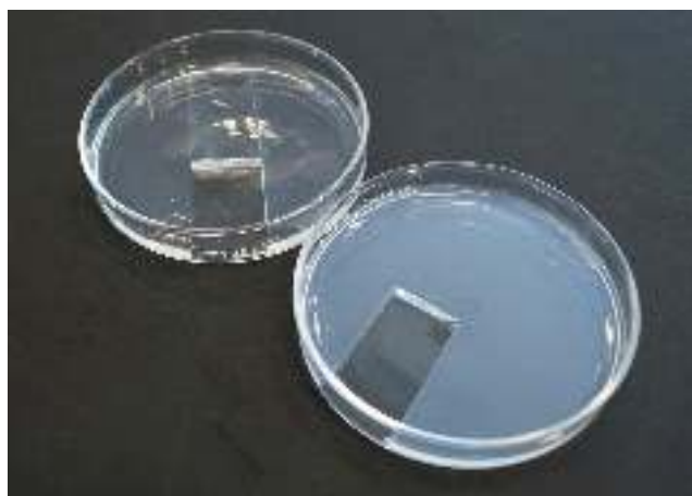
Fig. 3. Gellan gum (left) and agarose (right) prepared at 2% (w/v).
