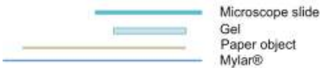
Fig. 6. Schematic diagram of gel application for local stain reduction.
