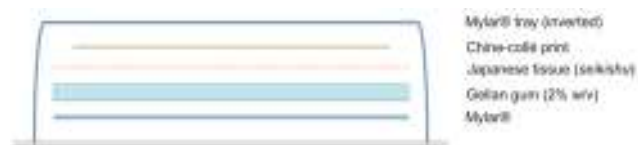
Fig. 12. Schematic diagram of arrangement for overall washing with a sheet of gellan gum.
