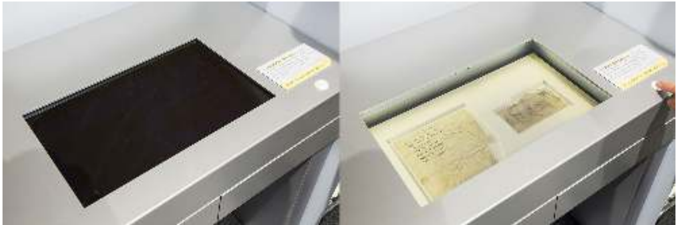
Fig. 23. Anthrax Letter case, on left, in the off state and on right, where push button activates SmartGlass.
