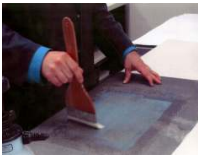
Fig. 4. Brush apply adhesive through a screen.
