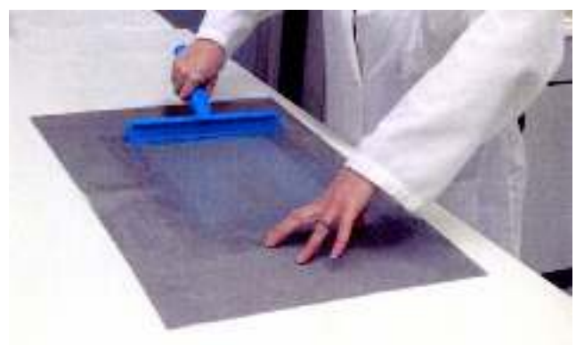
Fig. 5. After brush-applying adhesive, squeegee for even consistency.
