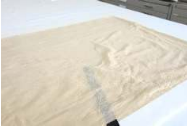
Fig. 9. Jeff Peachey's Carbon Fiber Lifter used to remove a fabric lining from a poster.
