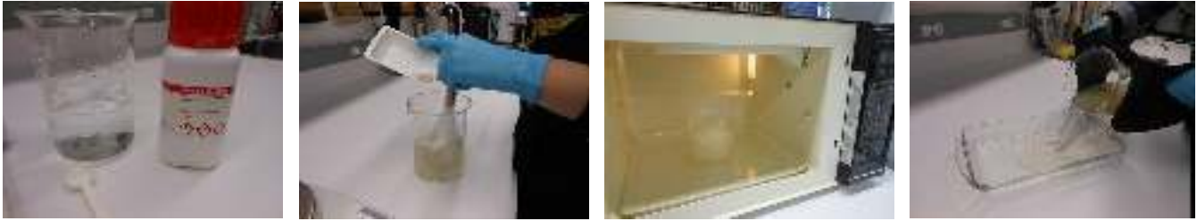
Fig. 3. Preparation of gellan gum gel.
