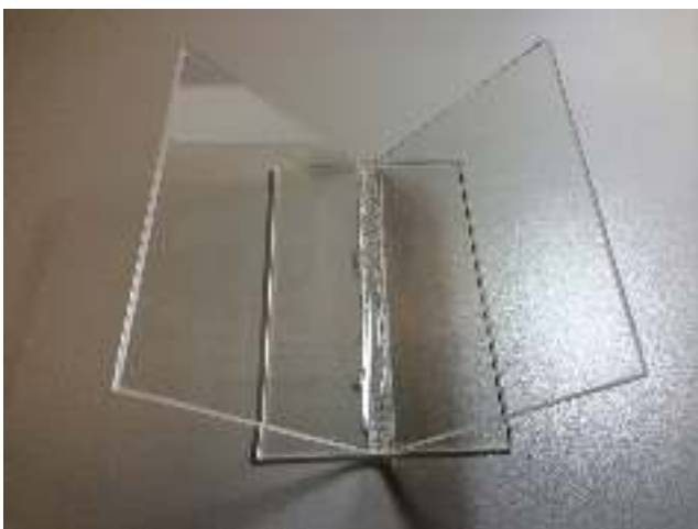
Fig. 5. One of the custom RBML Plexiglas cradles glued with quick and easy Plexi paste. The cradles survived travel to Germany and home using this paste.
