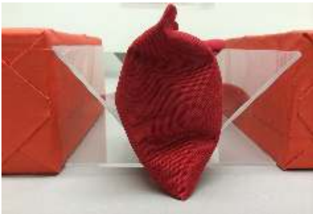
Fig. 4. After gluing out Plexi make sure to dry underweight in the fume hood.
