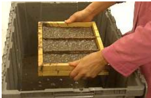
Fig. 17. Sheet forming during Trial 3, showing the gray and coarse textured pulp on the Japanese papermaking mould.
