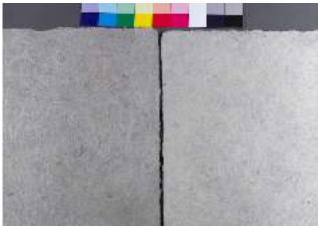
Fig. 22. Paper samples made from the pulp shown in figure 21, washed and beaten once (left); and three times (right).
