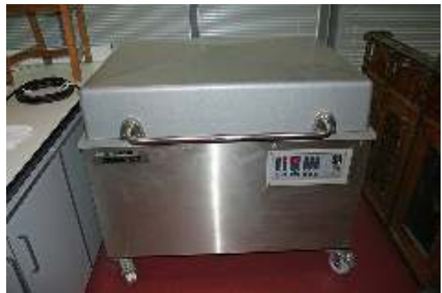
Fig. 10. Audionvac 401H vacuum m/c.
