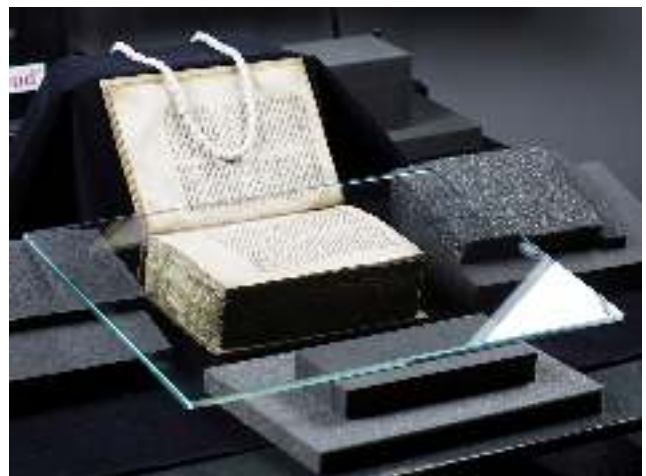
Fig. 16. A regular copy stand with 90–110 degree opening.
