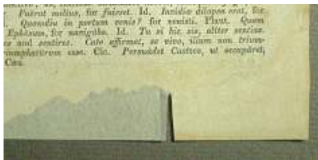
Fig. 2. Left: a fill made from two layers of uncoated Japanese paper laminated with dilute wheat starch paste. Right: a fill made from two layers of the same Japanese paper, coated with a solution of kaolin clay, calcium carbonate, and watercolor prior to mending
