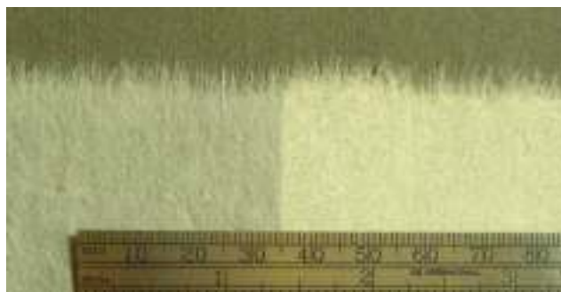
Fig. 1. Uncoated and coated Japanese paper with a water-torn edge
