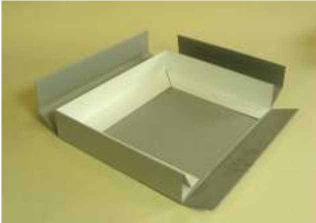
Fig. 6. This custom-made, corrugated drop-front box has aluminum-reinforced walls and corners. Two sheets of E-flute board are being used in perpendicular directions.
