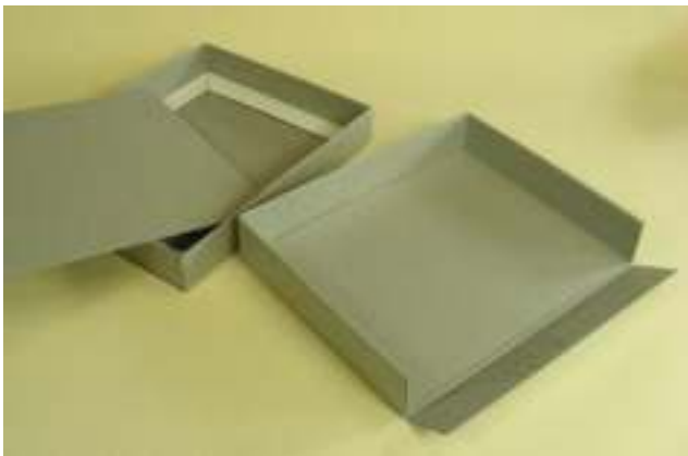
Fig. 7. The bottom of the drop-front corrugated box is assembled with three aluminum walls and minimal adhesive. The cover, made in the same way, has four aluminum walls and corners.
