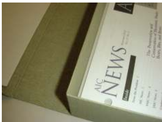
Fig. 2. This thin aluminum wall, laminated with acid-free paper and covered with starch-filled buckram, measured 0.045 in. thick, whereas a double wall of binders' board would have been 0.140 in. thick and weighed much more.
