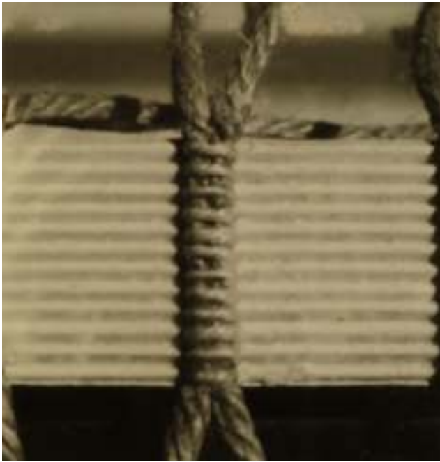
Fig. 5b. Example of two cords sewn as one, found in most printed books surveyed. Courtesy of Tamara Ohanyan
